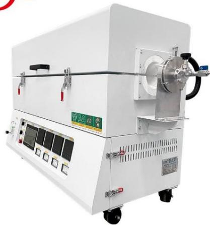
The GWL-KQGA series 1000°C high-temperature tubular furnace, as shown in the figure, integrates the control system and furnace chamber into a single design. The furnace lining uses high-purity alumina fiber and vacuum-formed fiber-reinforced lightweight board material.
